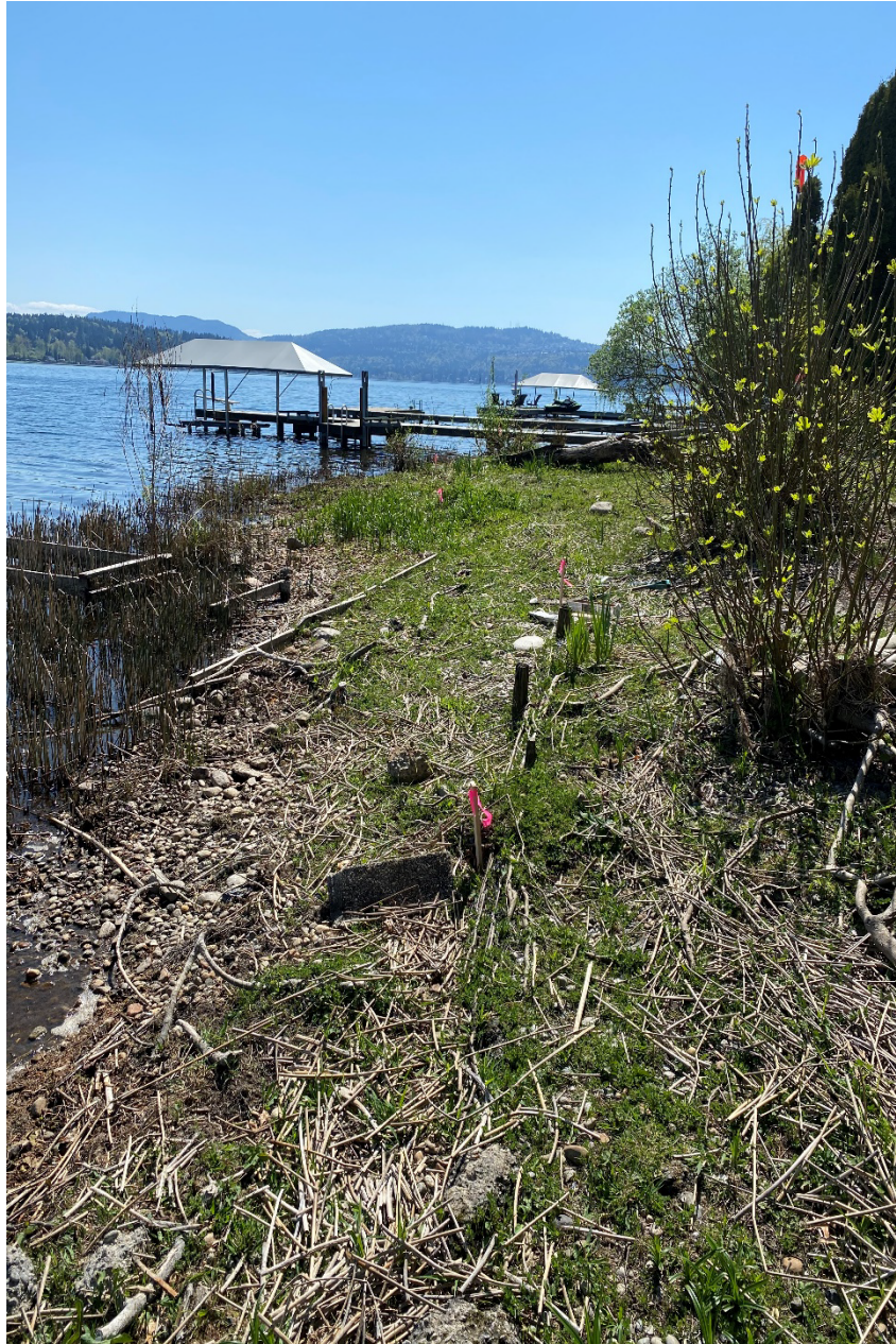
Typical view of OHWM (pink flags) looking south. Note pruned fig tree just above OHWM at right and larger exposed rocks with bulrush below OHWM at left.
