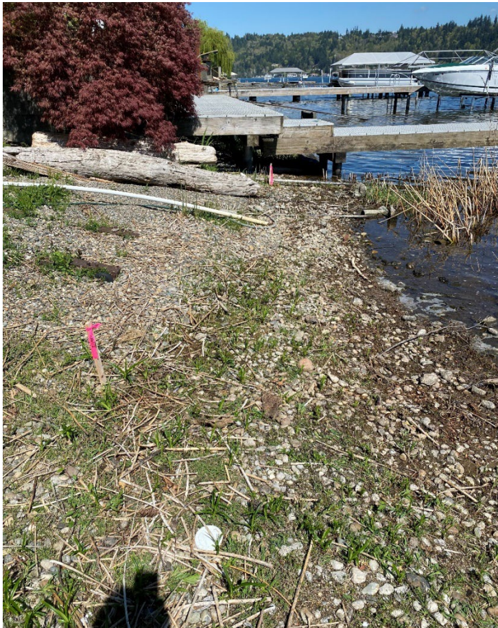
Typical view of OHWM (pink flags) looking north. Note Continuation of gravel beach above OHWM.
