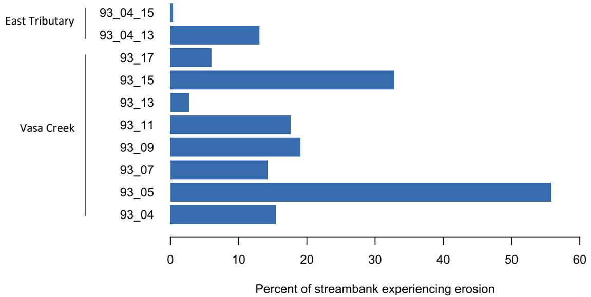
**Figure B-15. Percent of each OSCA-surveyed stream reach in the Vasa Creek Subbasin that is experiencing erosion.**
