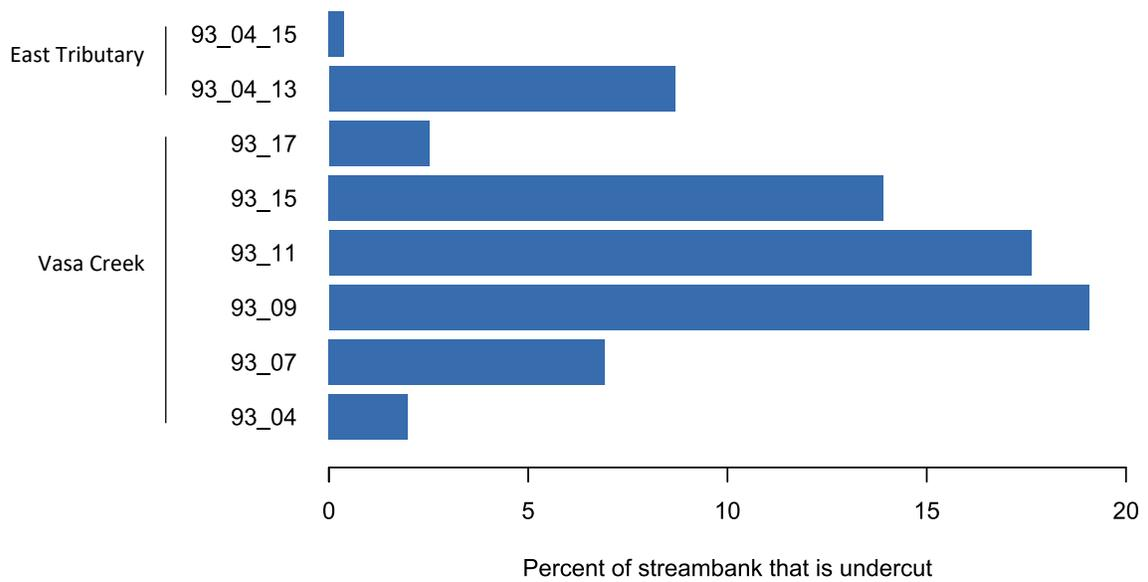
**Figure B-16. Percent of each OSCA-surveyed stream reach in the Vasa Creek Subbasin that has undercut streambanks. Mainstem Reaches 5 and 13 are omitted as they did not have undercut banks.**
