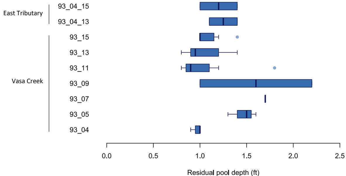
**Figure B-11. Boxplot of residual pool depths in OSCA-surveyed stream reaches of the Vasa Creek Subbasin. Mainstem Reach 17 is omitted as no pools were observed at the time of the survey.**
