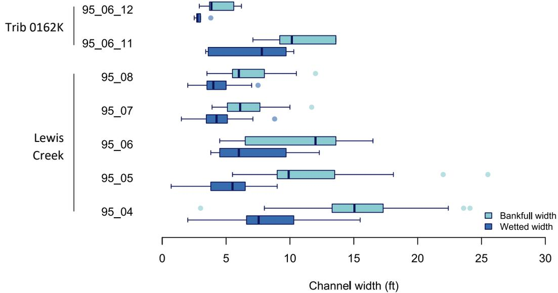
**Figure B-1. Boxplot of the wetted and bankfull channel widths for stream reaches in the Lewis Creek Subbasin that were surveyed under a Level 1 protocol.**
