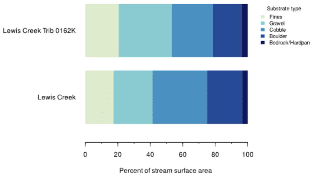
Figure 36. Substrate Composition of Riffle Habitat in Surveyed Reaches of Lewis Creek
