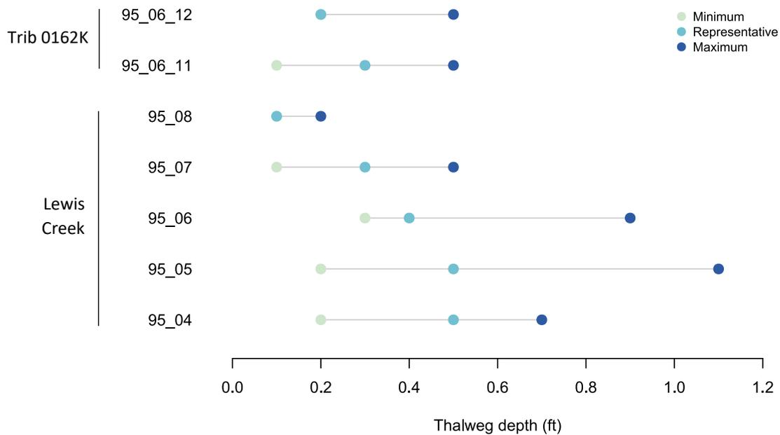
**Figure B-2. Dumbbell plot of wetted stream depths for stream reaches in the Lewis Creek Subbasin surveyed under a Level 1 protocol. Points represent the median value for the minimum, representative, and maximum depth for each reach.**
