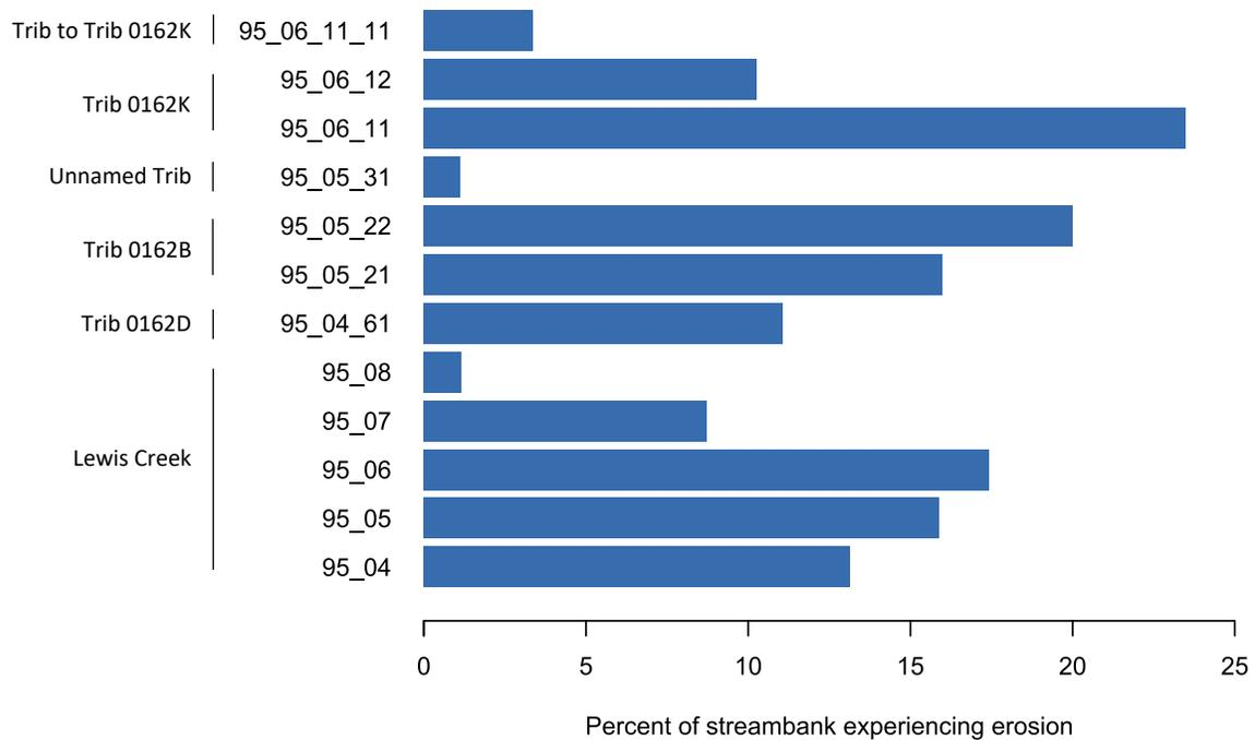
**Figure B-9. Percent of each surveyed reach in the Lewis Creek Subbasin that is experiencing erosion. Omitted reaches had no erosion.**
