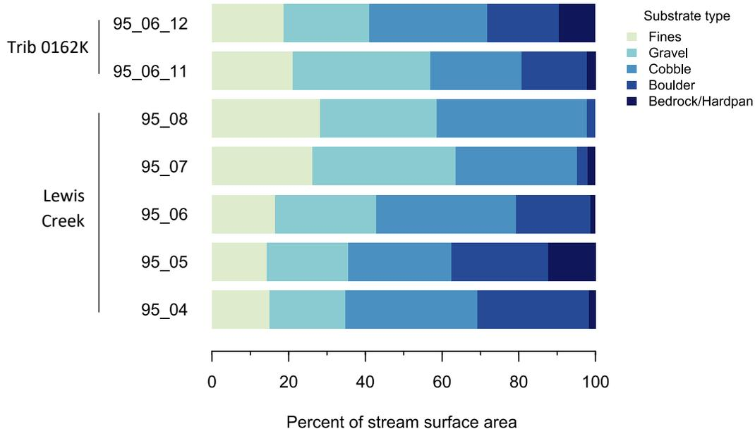
**Figure B-7. Substrate composition of riffle habitat in stream reaches of the Lewis Creek Subbasin surveyed under a Level 1 protocol, determined by visual estimation.**
