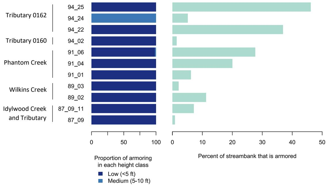
**Figure B-20. Multi-panel bar graph showing the percent of the streambank that is armored as well as the proportion of armoring in each armoring height class for each surveyed reach in the lesser tributaries to Lake Sammamish. Omitted reaches have no streambank armoring.**
