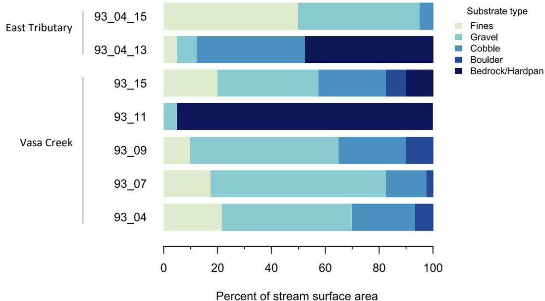
**Figure B-13. Substrate composition of riffle habitat in the Vasa Creek Subbasin, determined by visual estimation at representative stream cross-sectional profiles. Profiles were not taken in Reach 5 or 17.**
