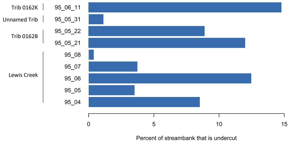
**Figure B-10. Percent of each surveyed reach in the Lewis Creek Subbasin with undercut streambanks. Omitted reaches had no undercut banks.**
