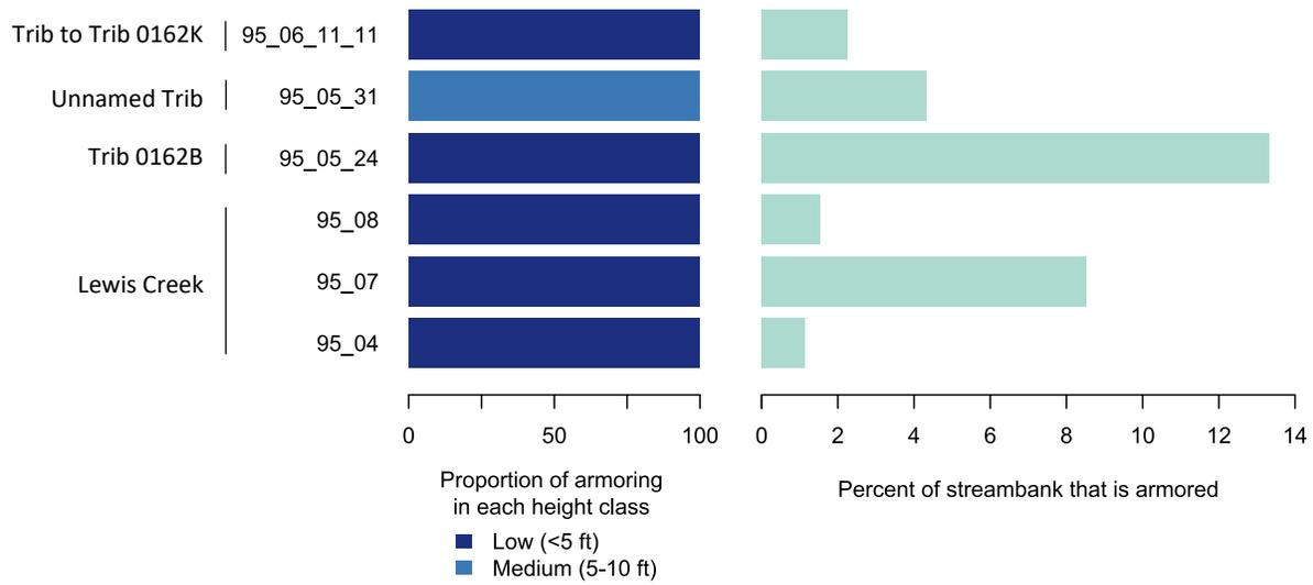
**Figure B-8. Multi-panel bar graph showing the height and proportion of armoring in each surveyed stream reach in the Lewis Creek Subbasin. Omitted reaches had no armoring.**
