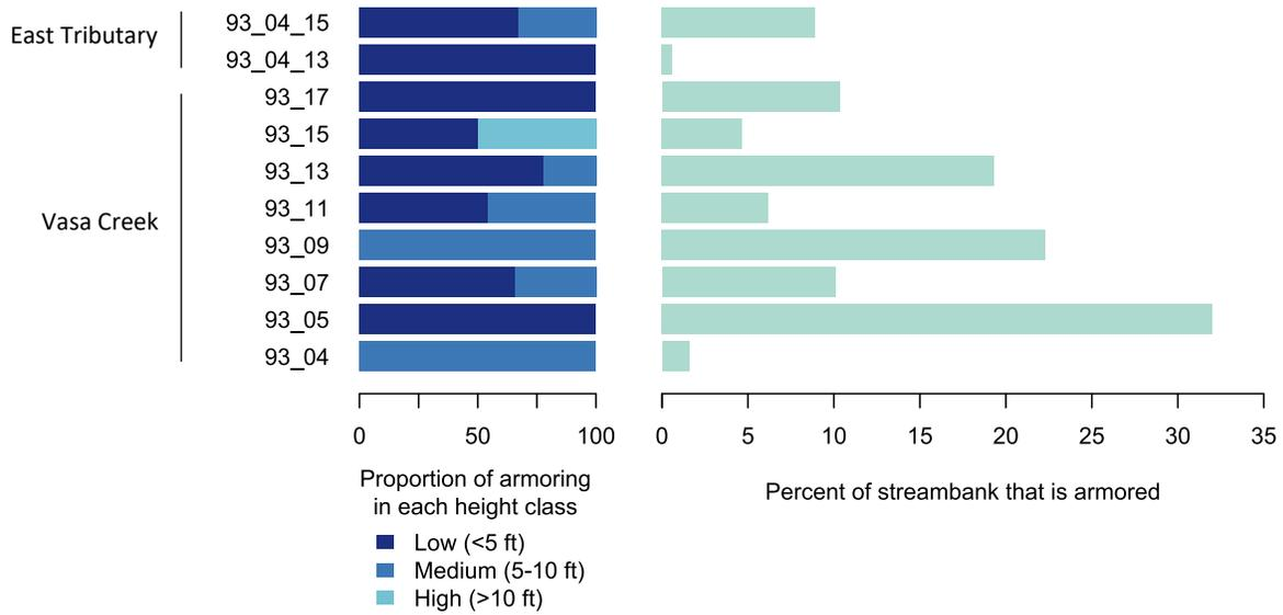
**Figure B-14. Multi-panel bar graph showing the percent of each OSCA-surveyed stream reach in the Vasa Creek Subbasin that is armored as well as the proportion of armoring in each armoring height class.**
