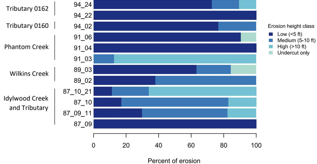
**Figure B-23. Proportional bar chart showing the percent of erosion falling into each height class.**
