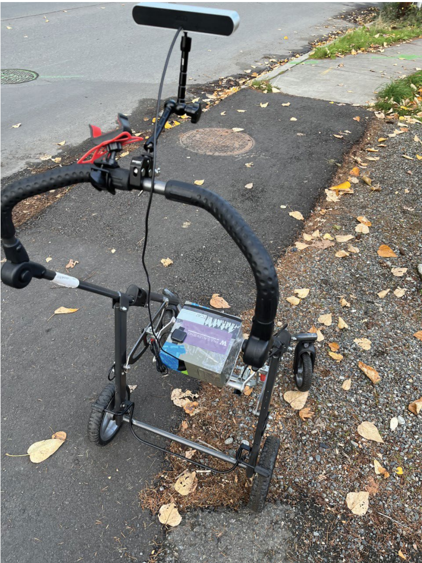
Part of the walking audits includes the use of a computer mounted on wheels that takes video of sidewalks and identifies potential hazards.
