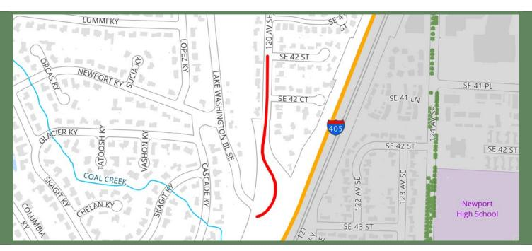
**Description:** This project would install up to four (4) new LED streetlights along 120th Avenue SE entering Greenwich Crest. On-going electricity costs would be paid for by the city. Actual locations would need to be examined further for feasibility. Streetlight location subject to adjacent homeowner approval.
