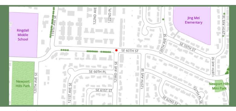
**Description:** This project would install new pedestrianactivated flashing system at the existing crosswalk over SE 60th Street and 123rd Avenue SE. Flashing beacons would be added on each side of the street. The proposed project would include associated street lighting upgrades.
