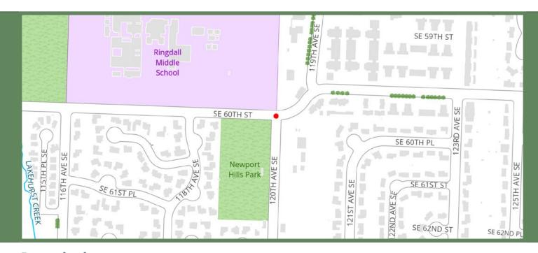
**Description:** This project would install new pedestrianactivated flashing system at the existing crosswalk over SE 60th Street and 123rd Avenue SE. Flashing beacons would be added on each side of the street. The proposed project would include associated street lighting upgrades and a new curb ramp on north side of street.
