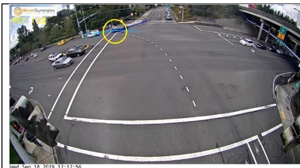
An Eastbound right-turning vehicle turning into a farther lane and crossing the conflict 1.22 seconds after the Westbound left turning vehicle
