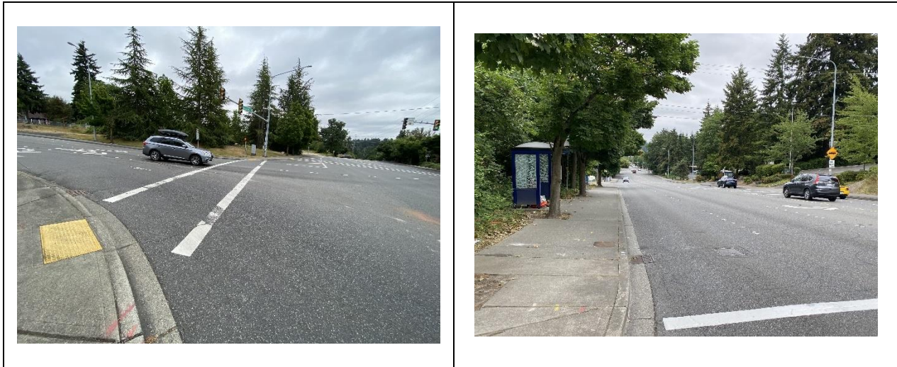
Figure 7 – Left: of SE Newport Way at Factoria Blvd, looking south, showing the wide crossing distance and standard transverse crosswalk markings. Credit: City of Bellevue. Right: Picture of Factoria Blvd, looking north on the west side of the street, showing the transit stop near the high school that was noted as frequently experiencing overflow of waiting riders. Credit: City of Bellevue.
