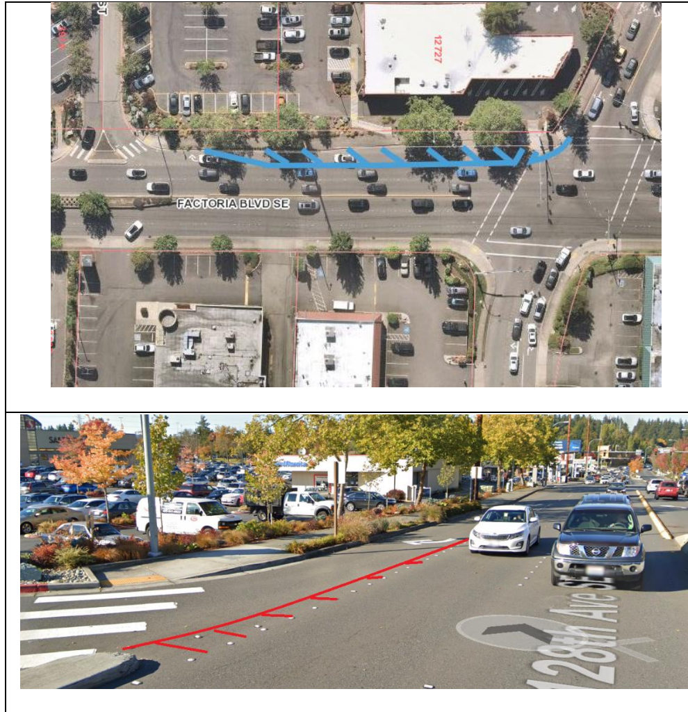
Figure 10 – Top: Concept sketch of dropped southbound right turn lane south of SE 38th St. Credit: City of Bellevue. Bottom: Concept sketch of updated turn lane channelization markings. Credit: City of Bellevue.
