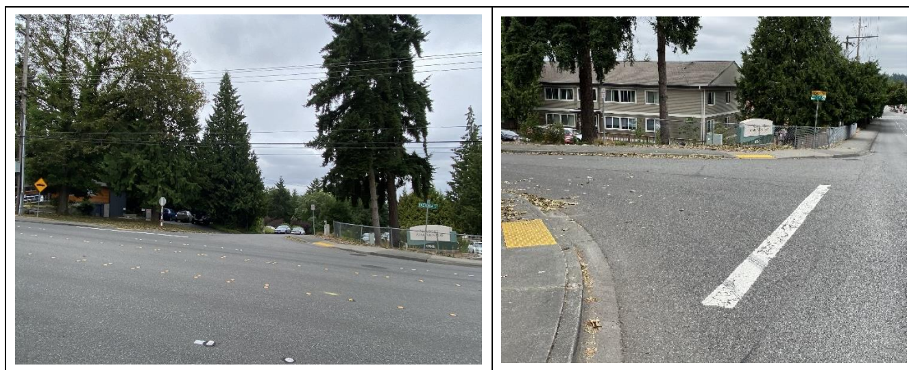
Figure 8 – Left: Picture of Factoria Blvd, looking west towards SE 42 nd St, showing a potential location for an uncontrolled marked crossing. Credit: City of Bellevue. Right: Picture Factoria Blvd at SE 42 nd , showing the placement of the stop bar in front of the curb ramps and no marked crosswalk. Credit: City of Bellevue.
