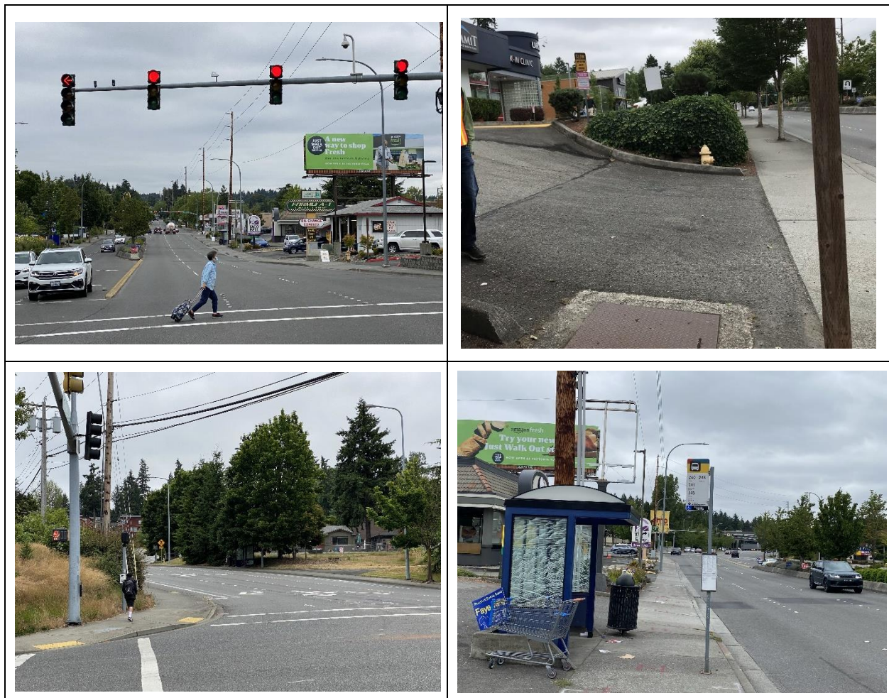
Figure 6 – Upper Left: Picture of Factoria Blvd, looking south at the 3700 Block, showing the median divided cross section at a signalized intersection. Credit: Complete Streets Bellevue. Upper Right: Picture of Factoria Blvd, looking south near SE 38 th St, showing driveway access to the street and limited visibility of the sidewalk due to vegetation. Credit: City of Bellevue. Lower Left: Picture of Factoria Blvd at SE Newport Way, looking east, showing the intersection, wide curb radii, and crossing distance. Credit: City of Bellevue. Lower Right: Picture of Factoria Blvd, looking south near 3711 Factoria Blvd, showing a transit stop constrained by two driveways. Credit: City of Bellevue.
