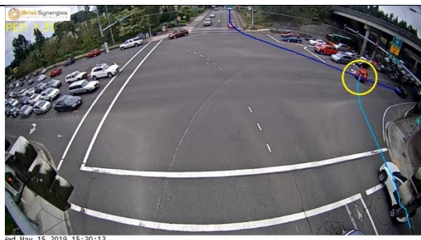
A Westbound right-turning vehicle turning 2 lanes away and crossing the conflict 1.31 seconds after the Westbound left-turning vehicle turning into a farther lane
