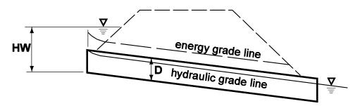
**Inlet Control - Submerged Inlet**
