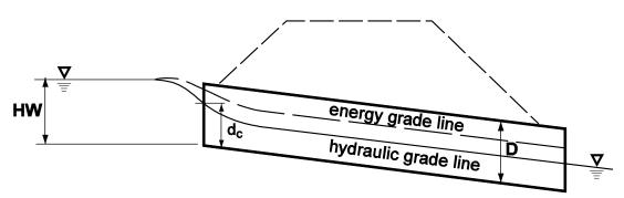
**Inlet Control - Unsubmerged Inlet**
