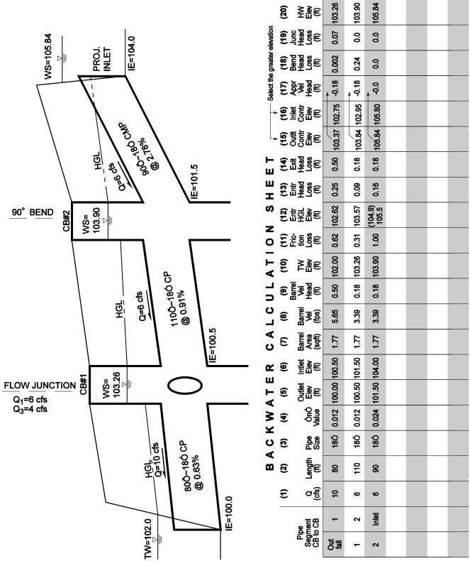
Figure 4.20 Bend Head Losses In Structures
