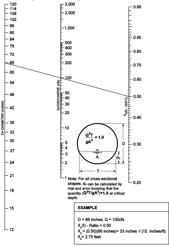
Figure 4.14 Critical Depth Of Flow For Circular Culverts
