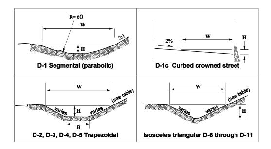
**Figure 4.4 Drainage Ditches - Common Sections**
