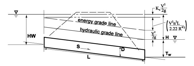
**Outlet Control - Submerged Inlet and Outlet**
