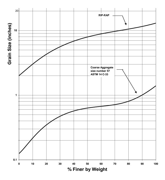
Figure 4.2 Riprap/Filter Example Gradation Curve
