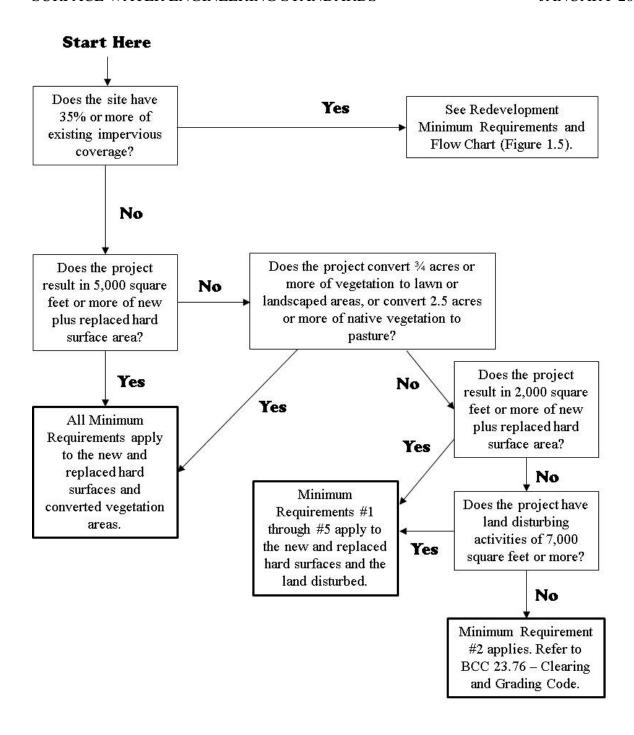
Figure 1.4 - Flow Chart for Determining Minimum Requirements for New Development Projects
