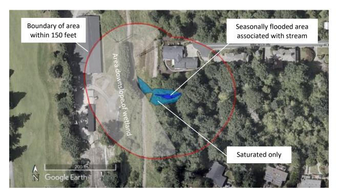
Figure EB05-2. Hydroperiods and 150-foot area for Wetland EB05 – H1.2, S2.1, S5.1
