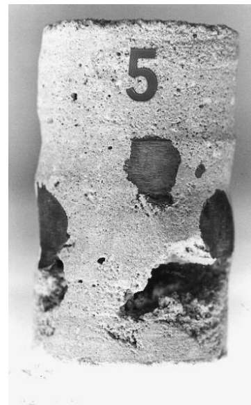
Shotcrete Cores: Grades 1 – 5 (Top Left to Bottom Right)
