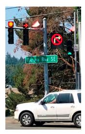
turns red. The signals are only activated when a bike is present – either by a loop sensor in the pavement or by a rider pushing a button on a post by the curb – so impacts to turning vehicles are limited.
