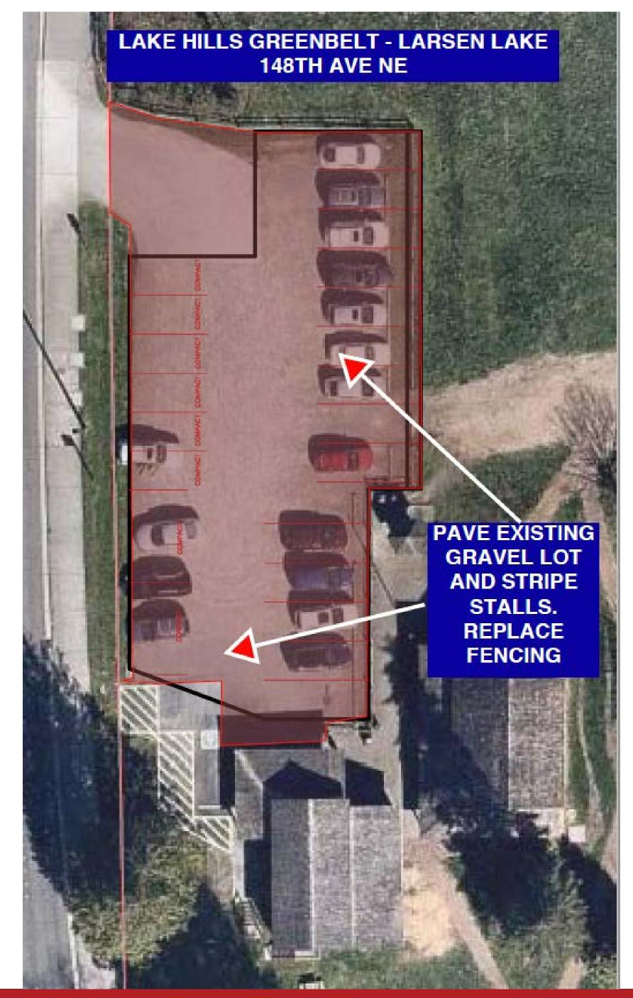
**Description:** This project would pave the existing parking area at Larsen Lake, including site drainage, pavement, striping and new fencing.
