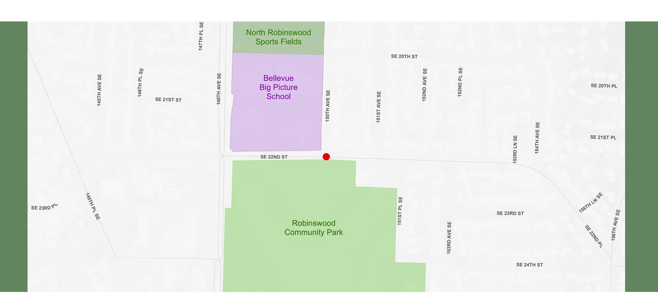
**Description:** This project would install a new marked crosswalk and a new rapid rectangular flashing beacon (RRFB) at SE 22nd St and 150th Ave SE. Project would construct curb ramps on both sides of the street and add a sidewalk connection to the Robinswood Park parking lot and adjacent walkway.
