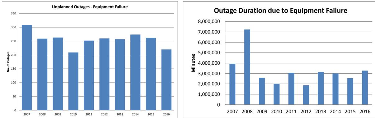
**Figure 10: Outage Data for Bellevue for Equipment Failure (Excluding Major Events)**
