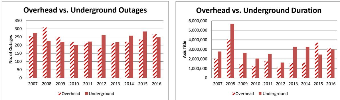
**Figure 14: Outage Data for Overhead and Underground Systems (Excluding Major Events)**
