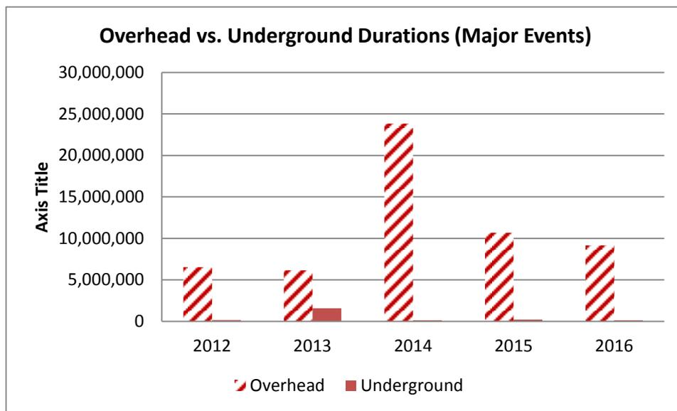
**Figure 15: Outage Duration for Overhead and Underground Systems (Major Storms Only)**
