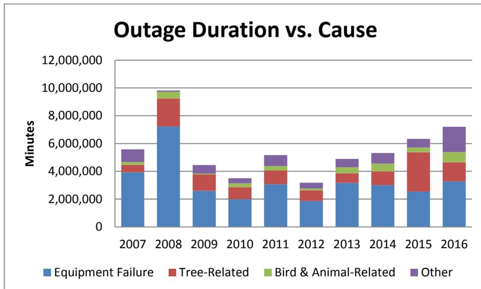
**Figure 9: Outage Duration vs. Cause**
