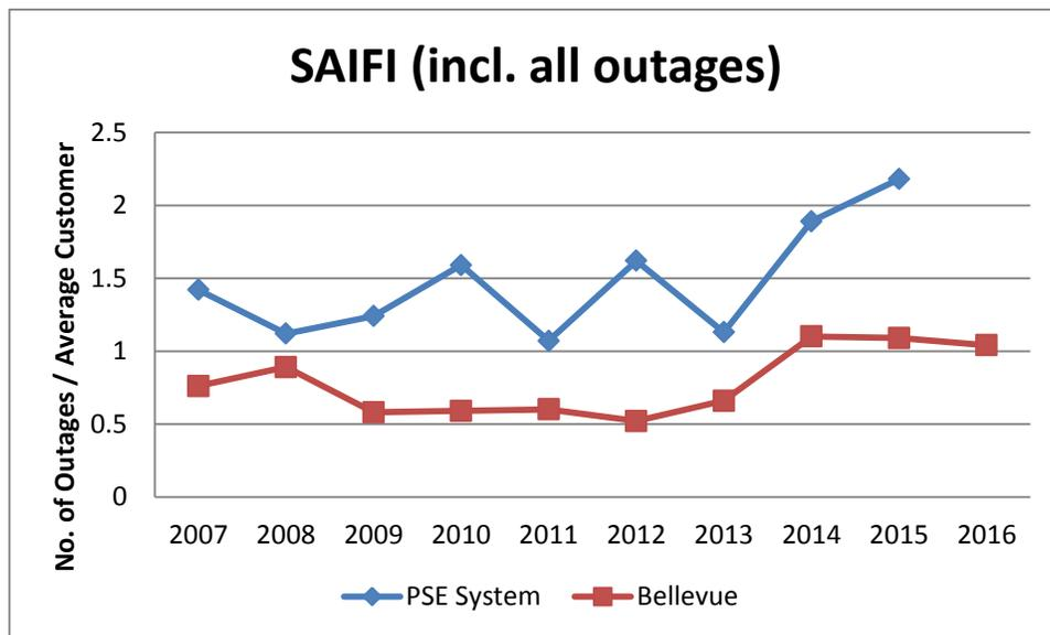
**Figure 3: SAIFI Metric for Planned and Unplanned Outages (Including major events) for Bellevue and PSE<sup>1</sup>**
