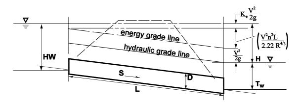
**Outlet Control - Submerged Inlet and Outlet**
