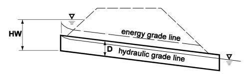
**Inlet Control - Submerged Inlet**
