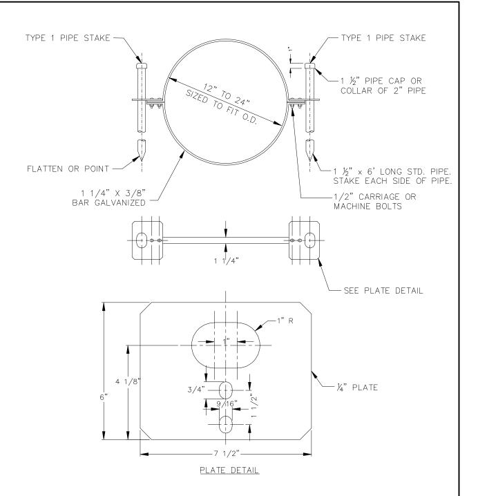
1. ALL PIPE STAKES, HARDWARE AND MATERIALS SHALL BE HOT DIPPED GALVANIZED AFTER FABRICATION.
