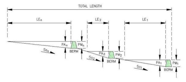
Figure 6.2. Schematic for calculating Bottom Length and Effective Total Depth for bioretention or pervious pavement on slopes where check dams (berms) are used. Refer to Table 6.6 for Rain Gardens and Bioretention Swales, and Table 6.8 for Pervious Pavement formulas.
