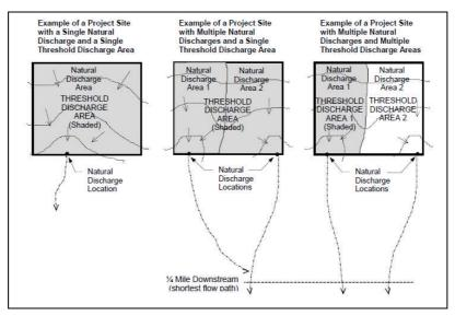
Figure 2.1 Threshold Discharge
