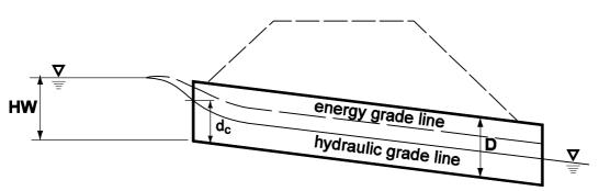
**Inlet Control - Unsubmerged Inlet**
