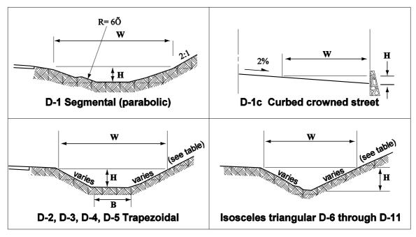
Figure 4.4 Drainage Ditches - Common Sections
