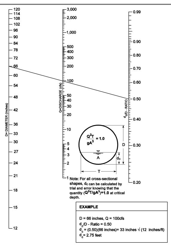
Figure 4. 14 Critical Depth Of Flow For Circular Culverts
