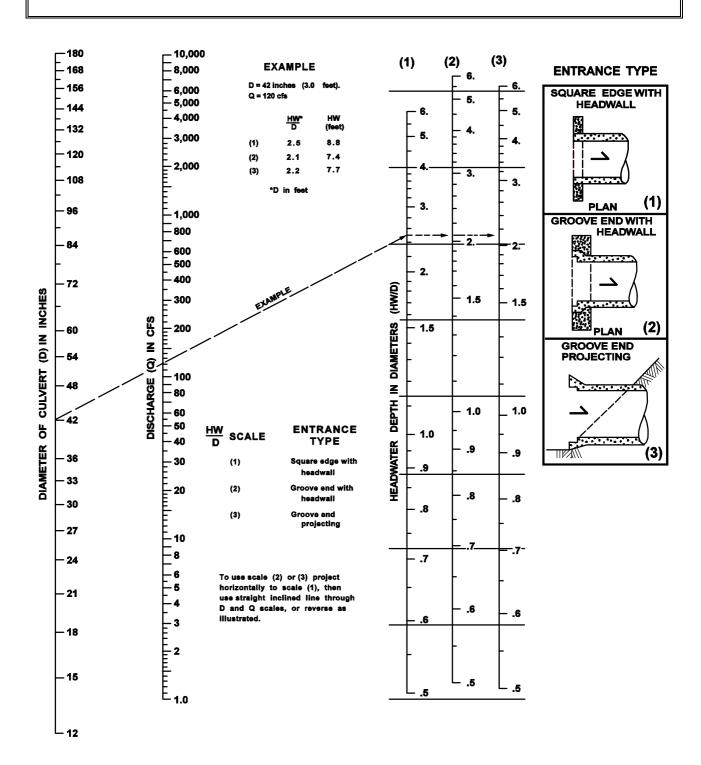
Figure 4.11 Headwater Depth For Corrugated Pipe Culverts With Inlet Control
