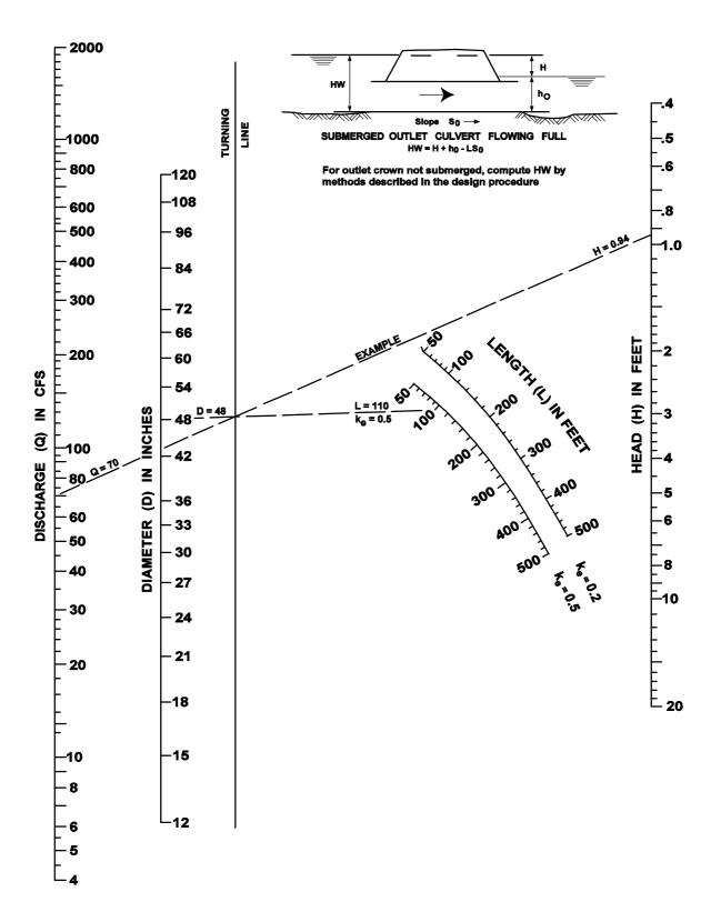
Figure 4. 13 Head For Culverts (Pipe W/"N"= 0.024) Flowing Full With Outlet Control
