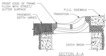
SET FRAME TO GRADE AND CONSTRUCT ROAD AND CURB TO BE FLUSH AT FRONT AND BACK OF FRAME.
