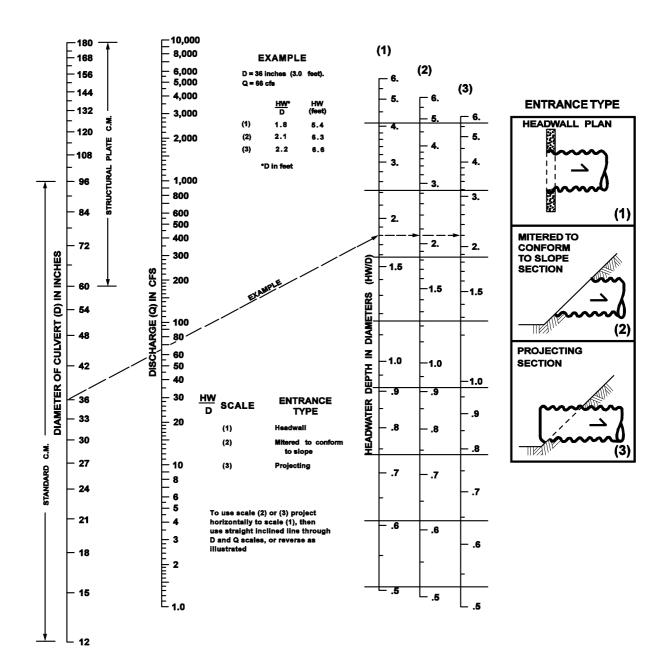
Figure 4.12 Head For Culverts (Pipe W/"N"= 0.012) Flowing Full With Outlet Control
