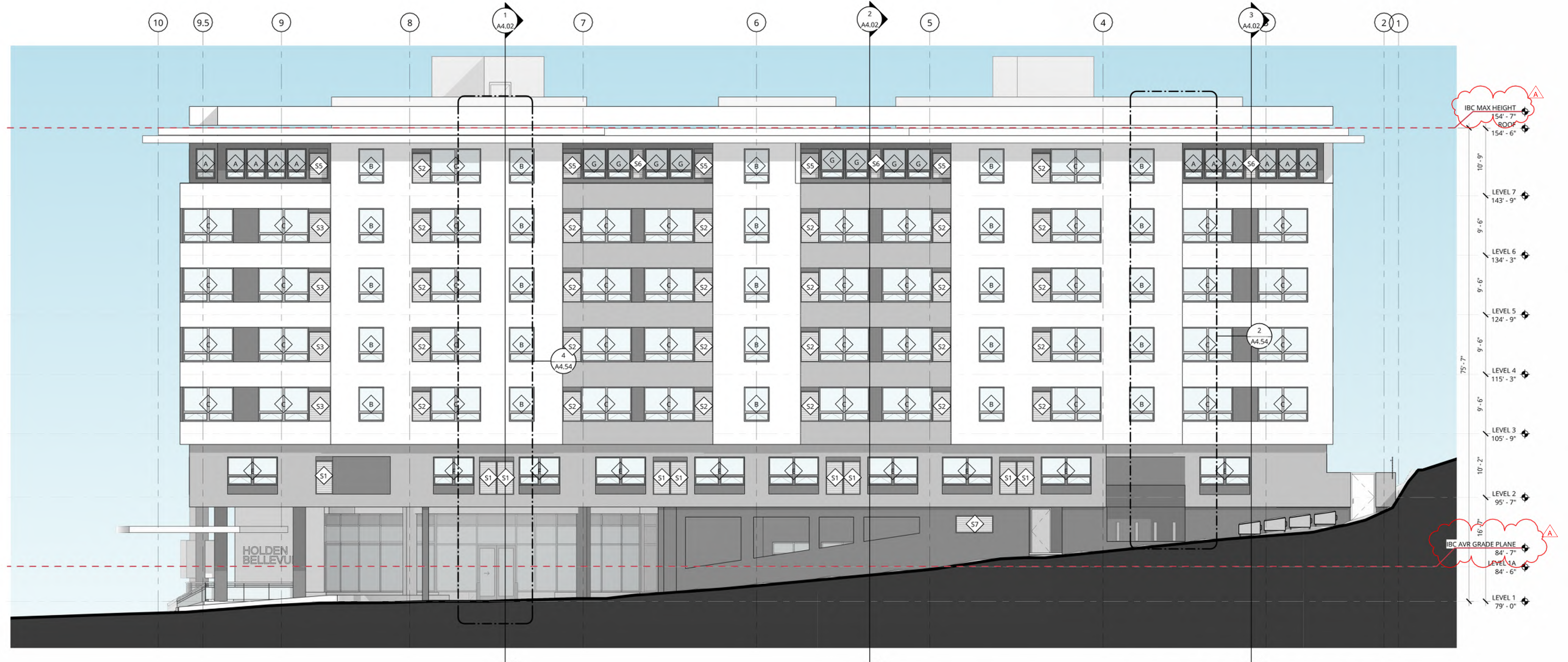
1 BUILDING ELEVATION NORTH 1/8" = 1'-0"
