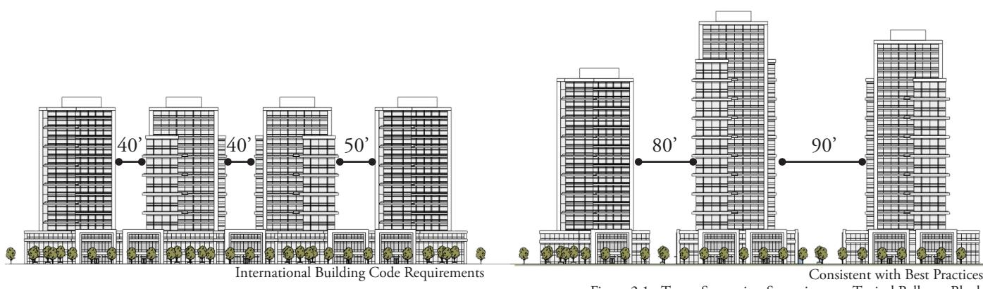
Figure 2.1 - Tower Separation Scenarios on a Typical Bellevue Block
