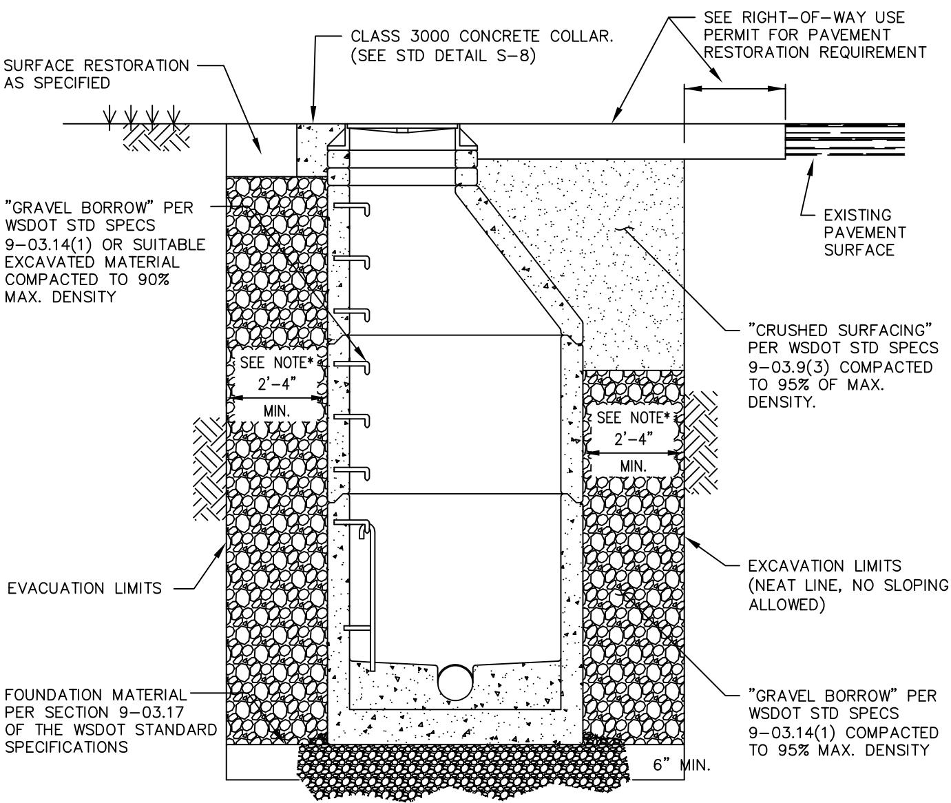
\* EXCAVATION LIMITS NEED TO INCREASE AS DEPTH INCREASES TO ACCOMMODATE LARGE SHORING BOXES, SLOUGH AND ROOM FOR A LARGER EXCAVATOR TO DIG DEEPER.
