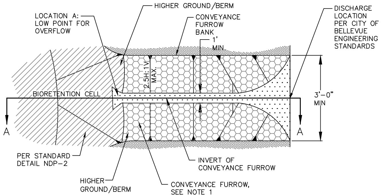
SECTION A – BIORETENTION CELL
