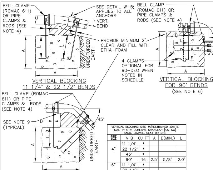
NO CHANGE IN PIPE DIRECTION OR DIAMETER SHALL OCCUR WITHIN 36 FEET OF THE VERTICAL BEND. BENDS, TEES, REDUCERS, ETC. BEYOND THE 36 FOOT LIMIT SHALL BE RESTRAINED BY STANDARD CONCRETE BLOCKING PER STD. DTL. W-1 & W-3. CONCRETE BLOCKING SIZES BASED ON:
