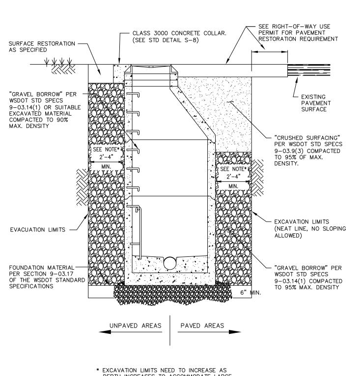
\* EXCAVATION LIMITS NEED TO INCREASE AS DEPTH INCREASES TO ACCOMMODATE LARGE SHORING BOXES, SLOUGH AND ROOM FOR A LARGER EXCAVATOR TO DIG DEEPER.
