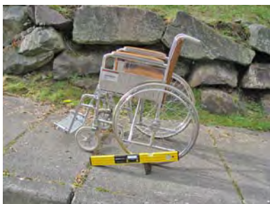
Sidewalk grade of 22% on 166th Avenue SE between Phillips Road and SE 39th Place.
