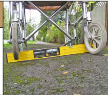
Example of 18 percent cross slope at NE 24th Street & 167th Avenue NE.
