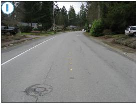
6 foot-wide shoulder on the east side of SE 161st Avenue SE accommodates parking, and the narrow sidewalk on the west side begins at NE 24th Street, but is an extremely short segment, ending shortly thereafter.
