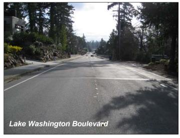
10<sup>th</sup> Street to 100<sup>th</sup> Avenue NE where not already complete. This is in conjunction with pedestrian project **S-318-S**, which calls for a 6 foot wide sidewalk and a 4 foot wide planter strip along the south side of Lake Washington Boulevard between NE 1<sup>st</sup> Street and 100<sup>th</sup> Avenue NE where not complete. This section of Lake Washington Boulevard provides access to Clyde Beach Park and Meydenbauer Beach Park as well as the Ground Zero Teen Center.
