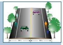
Diagram illustrating the desired dimensions of a shared bike shoulder facility.
