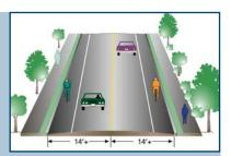
Diagram illustrating the desired dimensions of a designated bike shoulder with fog line facility.
