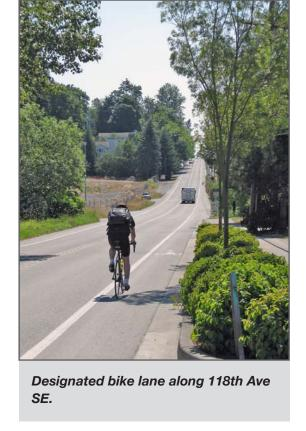
• Bicycle Lanes: As defined in WSDOT's Design Manual (Chapter 1020 Bicycle Facilities), a bike lane is "a portion of a highway or street identified by signs and pavement markings as reserved for bicycle use." Bike lanes provide bicyclists with their own lane designation along street corridors with high vehicular volumes or speeds. The following features of bicycles lanes increase the comfort of the average cyclist and the overall safety of the roadway:
