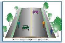
Diagram illustrating the desired dimensions of a wide outside lane, without a fog line.
