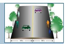
Diagram illustrating the desired dimensions of a shared wide outside lane.
