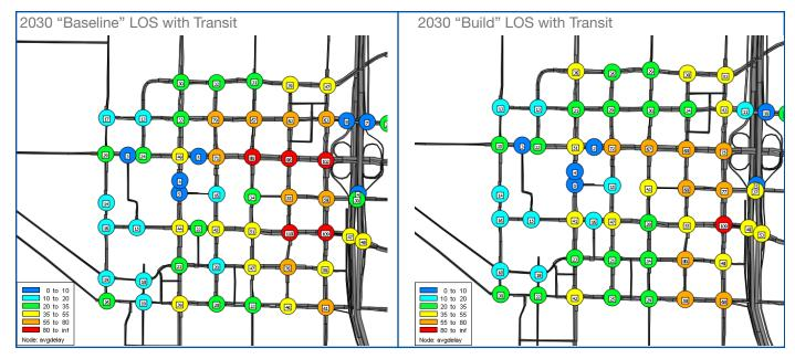
Figure 6. Dynameq Modeling Output - Vehicle Level-of-Service (Delay)
