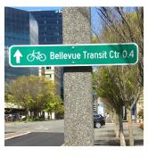
signage at decision points that identifies the direction and distance to specific destinations, and confirmation signage after the turn to point the bicycle rider in the right direction.
