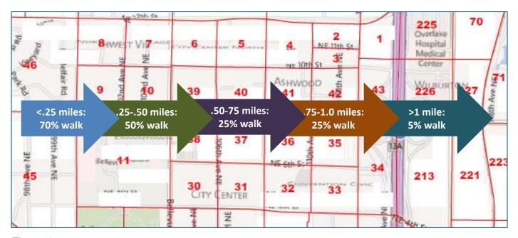
Figure 1. Distance Methodology for Internal Walk Trip Calculation
