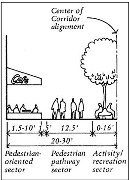
Figure 19. Building the Pedestrian Corridor by Halves
