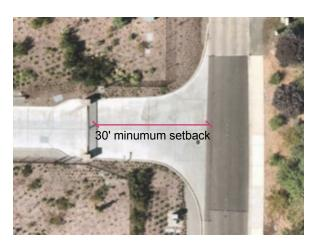
**Exception**: Automated gates equipped with Click 2 Enter or other authorized equipment that allows for operation of the gate by Fire and Police personnel from their vehicle are not required to be set back 30 ft. from the roadway edge of pavement provided the roadway is not an arterial, residential collector street or a street with lane markers.
