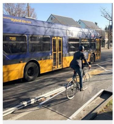
**Figure 3.** The new bus platform is installed on 108th Ave NE south of NE 2nd St. It is made of 300 interlocking plastic panels that snap together, allowing for its rapid installation.
