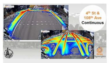
**Figure 19.** Heatmap from Brisk Synergies video intelligence algorithms depicting pedestrian crossings and motor vehicle turning movements at 108th Ave NE and NE 4th St.
