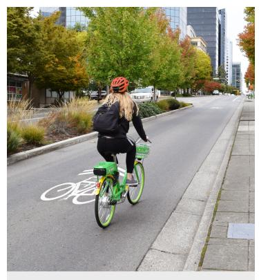
**Figure 10.** A person riding northbound in the marked shared lane north of Main St, where the travel lane is too narrow for a bike lane due to an existing planted median.
