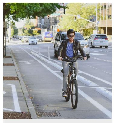
**Figure 8.** A person riding southbound in the bike lane south of NE 8th St, where Tuff Curb—a durable traffic safety product—provides physical separation for people on bikes.
