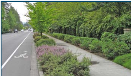
Example of a 6 foot-wide sidewalk and a 4 foot-wide planter at 140th Avenue NE and NE 1st Place.
