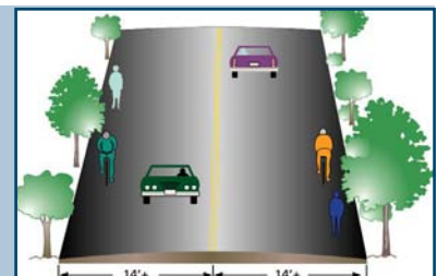
Diagram illustrating the desired dimensions of a shared wide outside lane.
