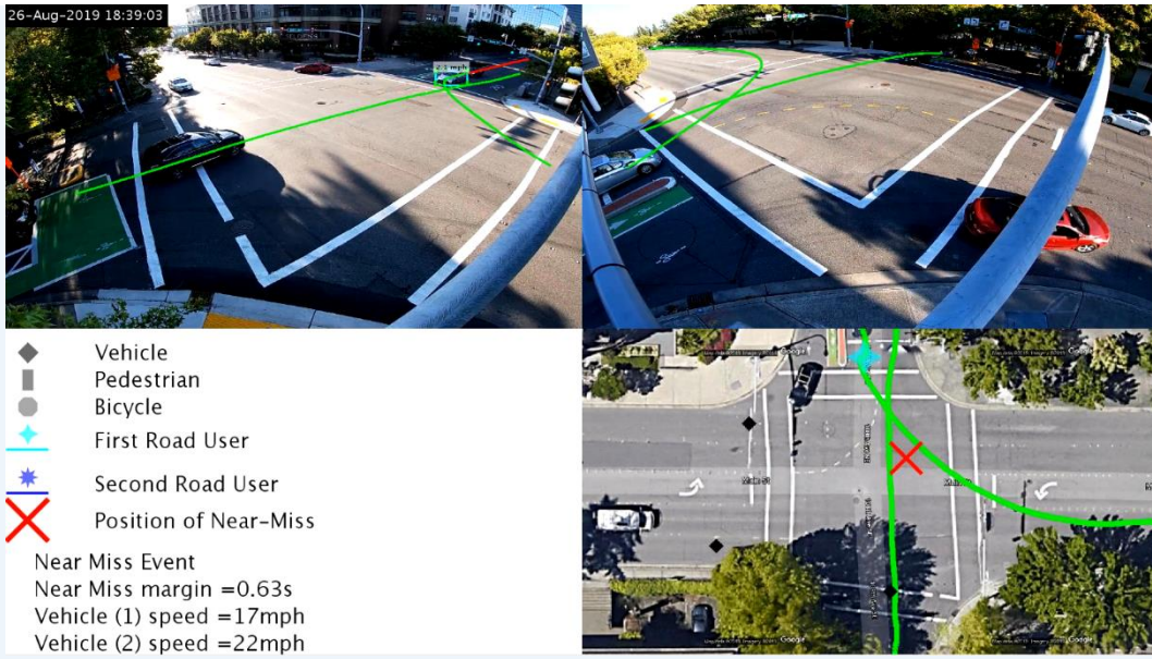
Figure 3. Shadows as a contributing factor to the conflicts shown above. Heavy shadowing of northbound vehicles could inhibit visibility to southbound left turning vehicles. Left turning vehicles are observed either failing to see oncoming vehicles or misjudging distance and speed. Once the through motion vehicle exits the shaded area the left turning vehicle has less than 3 seconds to react. The top right view is similar to the view that 108th southbound drivers have of the scene.
