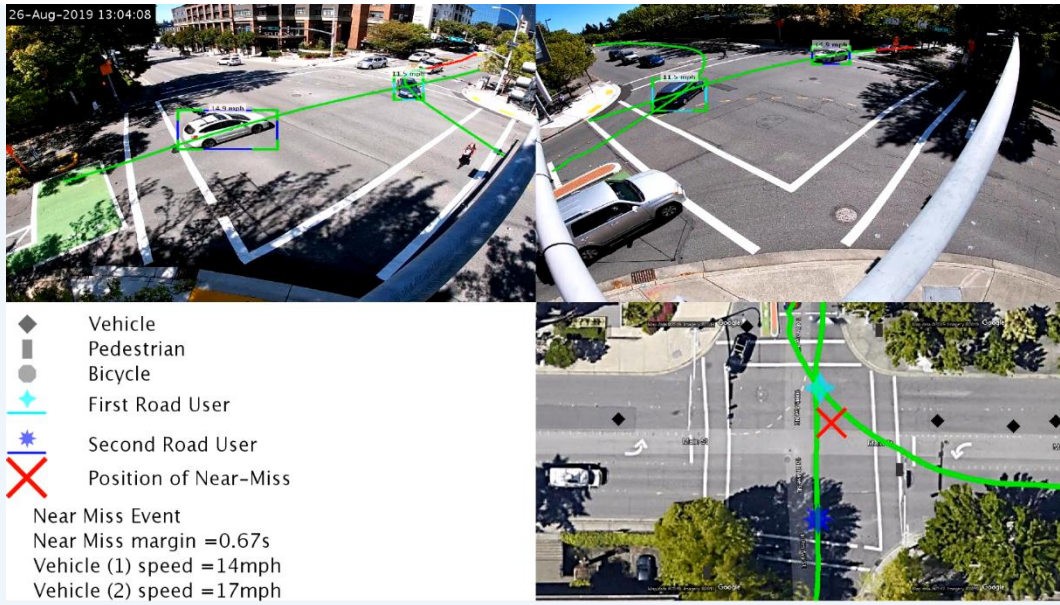
Figure 5. Three conflict participant near miss involving 108th southbound left vehicle, 108th northbound through vehicle, and southbound pedestrian in the East crosswalk. The left turning vehicle took a sharp left near a pedestrian to avoid being hit by a fast approaching through vehicle. The post-encroachment time between the two vehicles was only 0.67 seconds which is not enough time for either road user to stop.
