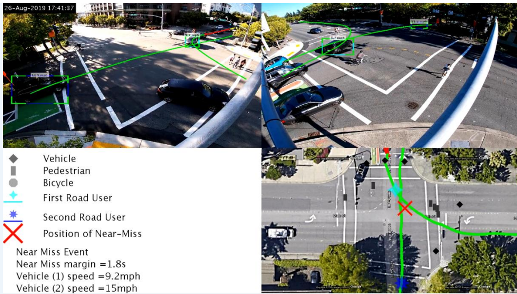
Figure 6. A second three conflict participant near miss involving 108th southbound left vehicle, northbound 108th through vehicle, and southbound pedestrian in the east crosswalk. In this case, the through moving vehicle on northbound 108th was occluded by a right turning vehicle of the same color. The left turning vehicle committed to the motion, blocking the through motion lane, but slowed down to avoid hitting three pedestrians crossing the street. The through moving vehicle quickly accelerated, then slowed to allow the left turning vehicle to clear the intersection.
