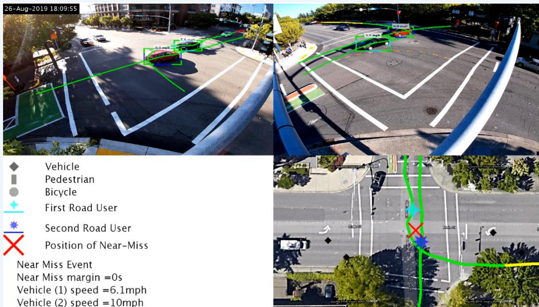
Figure 2. High risk near miss event on 108th SB left with 108th NB through. Vehicles almost collide, abruptly stop, and maneuver around each other to complete their motions. The top left and right views are the videos used for the study overlaid with the vehicle path information and vehicle speeds. The bottom left pane shows the conflict type, the post encroachment time (near miss margin), and the average vehicle speeds of each road user. The bottom right pane is a google maps overlay showing the paths each road user took, and the location of the near miss.
