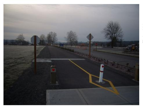
FIGURE 63 Bollards prevent unauthorized trail use but are easier to maneuver than dismount gates
