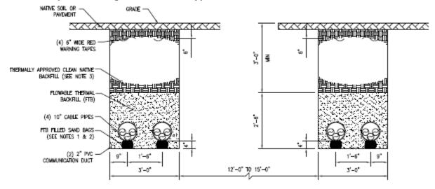
Figure 3-14 HPFF Typical Trench Detail
