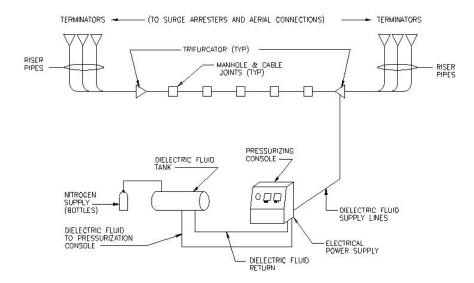
Figure 2-14 Typical HPFF Cable System
