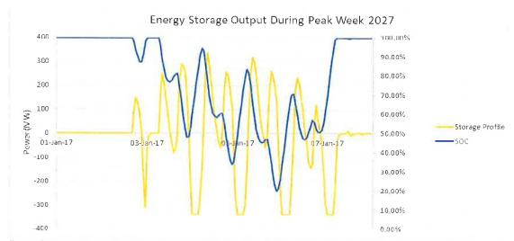
Figure 6: Output of the Complete Solution during the peak week, 338MW/3,679MWh (10.9-hour system)
