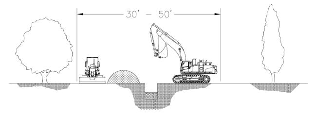
Figure 3-6: Off-road Construction
