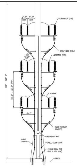
Figure 2-17 XLPE Double Circuit Single Shaft Transition Structure Schematic
