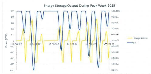
Figure 8: Output of the Interim Solution during the peak week, 365MW/2,394MWh (6.6-hour system)
