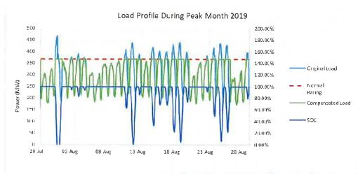
Figure 9: Performance over peak summer month, 365MW/2,394MWh (6.6-hour system)
