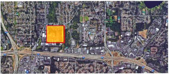
Figure 17: Indicative footprint of the Eastside storage solution red, single-level Interim Solution 59 acres, and yellow double-level Complete Solution, 49 acres
