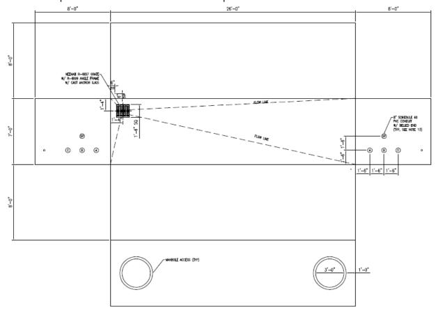
Figure 2-8 XLPE Vault Schematic
