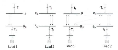
Figure 23: Rodial configuration left (dual circuit) and mesh configuration right
