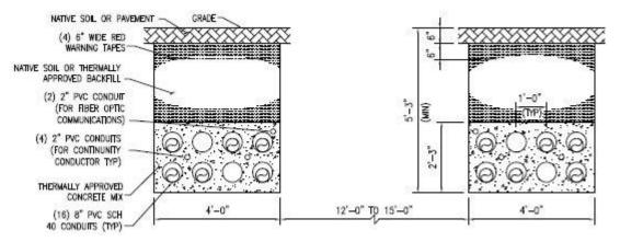
Figure 3-11 XLPE Typical Trench Detail
