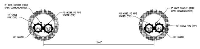
Figure 3-16 HPFF Typical Jack and Bore Detail
