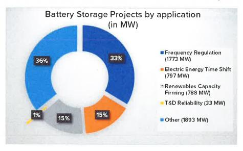
Figure 34: Battery Energy Storage Primary Applications
