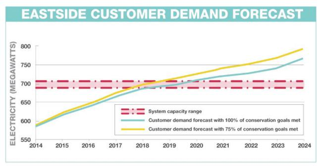
*Figure 4: PSE's graph shows customer demand exceeding system capacity in 2018.*<sup>2</sup>
