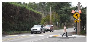
Example Rectangular Rapid Flashing Beacon system
