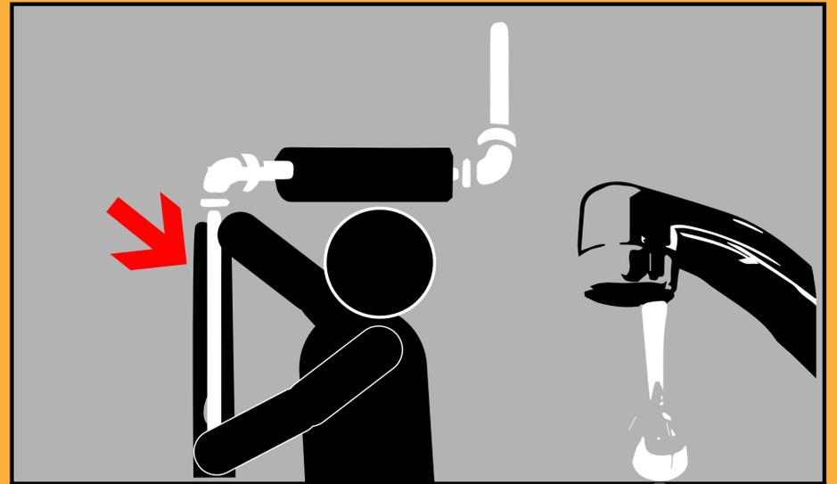
¡ASEGÚRESE QUE LAS TUBERÍAS INTERNAS Y EXTERNAS ESTÉN CUBIERTAS CON UN MATERIAL AISLANTE!
