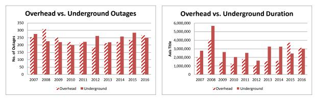
Figure 14: Outage Data for Overhead and Underground Systems (Excluding Major Events)
