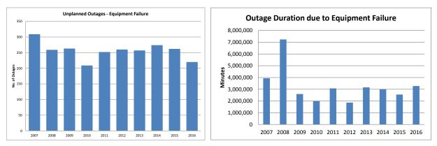
Figure 10: Outage Data for Bellevue for Equipment Failure (Excluding Major Events)
