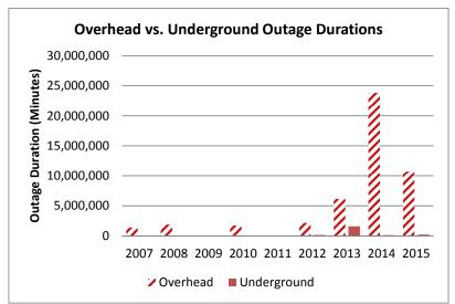
Figure 15: Outage Duration for Overhead and Underground Systems (Major Storms Only)
