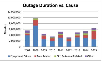
**Figure 9: Outage Duration vs. Cause**
