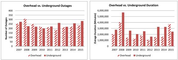
Figure 14: Outage Data for Overhead and Underground Systems (Excluding Major Events)
