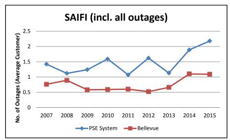
Figure 3: SAIFI Metric for Planned and Unplanned Outages (Including major events) for Bellevue and PSE
