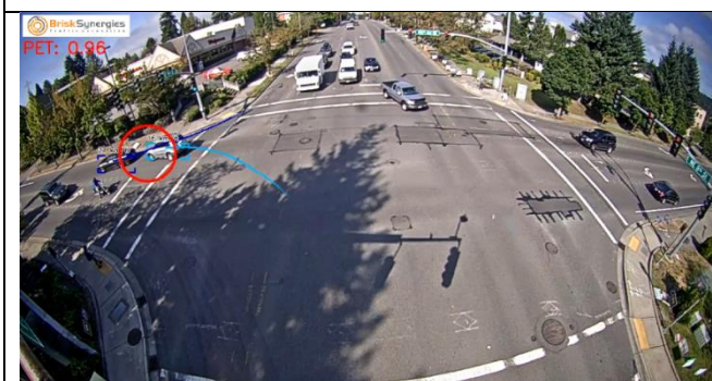
A westbound left turning vehicle tailgating an eastbound right turning vehicle 0.96 seconds behind
