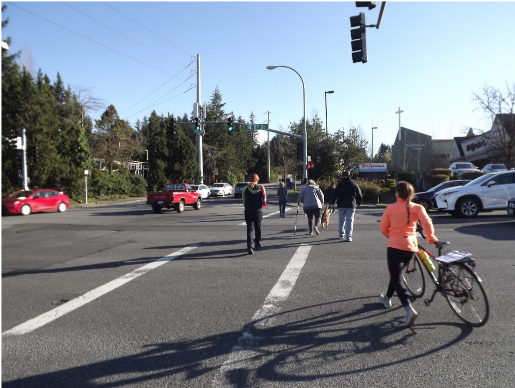
Left: Most of our group was still tens of feet removed from the other side of the crosswalk when the timer reached zero. Because this intersection is used by families, seniors, and people of different mobility levels, these crosswalk times should be lengthened to safely accommodate more people.
