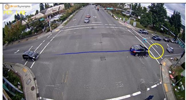
A pedestrian jaywalking out of phase and walking after a through driver by 1.42 seconds
