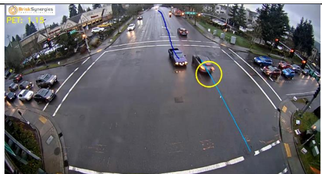
An eastbound left turning vehicle arriving at the conflict point 1 second after a westbound through vehicle
