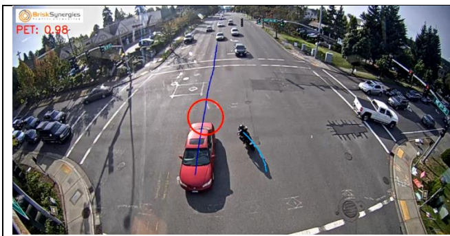
A westbound left turning motorcyclist arriving at the conflict point 0.98 seconds after an eastbound through vehicle
